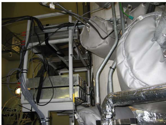
Figure 19 (Left) Detector arrangement in situ next to lagged bed and (right) circulation arrangement, with central baffle; arrow shows additional gas injection (Ingram et al., 2007).
