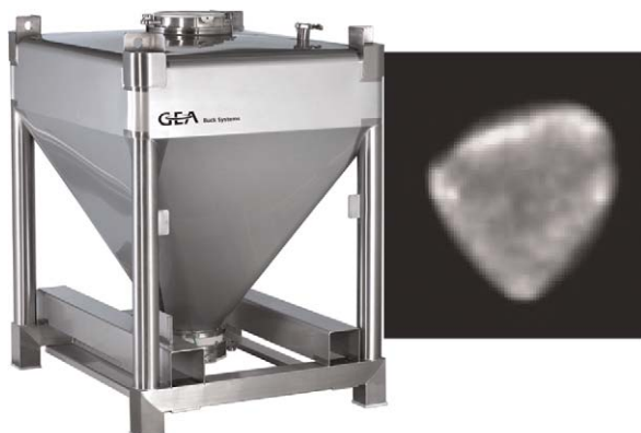
Figure 16 PET image (right) of dispersion of a pseudo drug substance within an excipient contained in a mixing vessel (left) (Armstrong et al., 2005).
